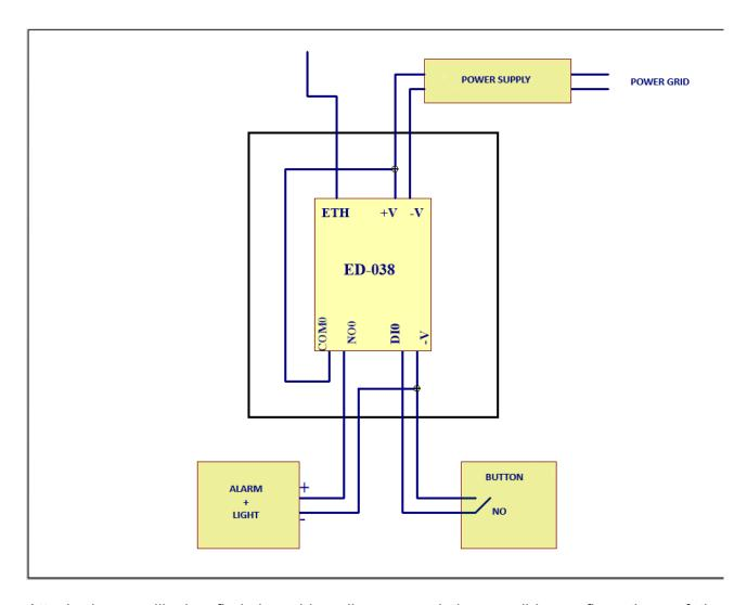
Attached you will also find the wiring diagram and the possible configurations of the Banshee Excel Lite alarm with integrated light and the button.
