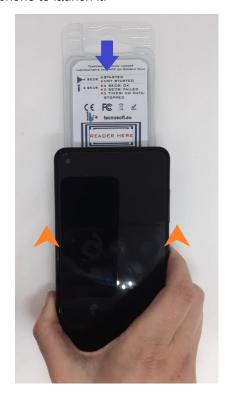
Place the data logger with the back facing upwards, the sensor is positioned under the word "READER HERE", slide the back of the phone upwards until you feel a vibration, at which point stop and wait for the screen to evolve.
